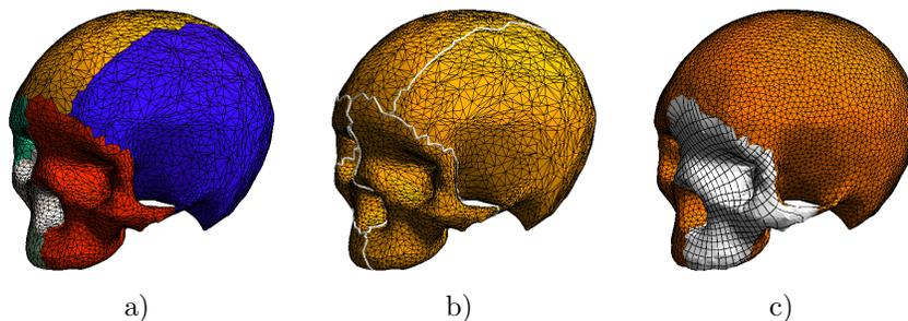
Figure 1: Remeshing algorithm for a skull geometry. a) Initial triangulation ( $G = 2$ ,  $NB = 0$ ), b) Remeshing of the lines at the interfaces between partitions, c) Computation of a harmonic map for every partition and remeshing of the partitions in the parametric space.
